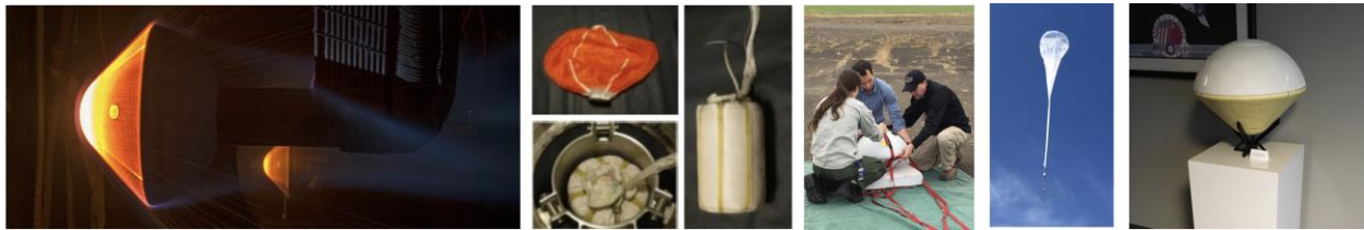
Figure 2: SpaceWorks' Heritage RED-Data2 and RED-4U STV Capsules. NASA Ames ARC Jet testing of RED-Data2 (left), RED-4U ballistic recovery system and high-altitude balloon test (middle), and automatic opening RED-4U mockup (right)
